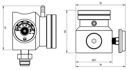
The Compact Demand Flow Regulator (CDFR) is engineered to provide a constant and precise flow of calibration gas directly to instruments on demand. Its compact design allows easy integration into portable and fixed gas calibration setups, ensuring accuracy and convenience in limited-space environments. Constructed with hard anodized aluminium for durability and chemical compatibility to certain reactive gases, the CDFR delivers reliable performance for both field and laboratory applications.
