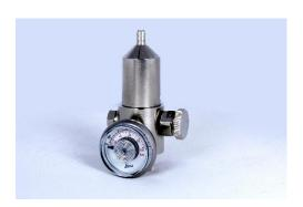
PUSH TYPE REGULATOR USED FOR CALIBRATION GASES AND INDUSTRIAL SAFETY MONITORS. THESE ARE AVAILABLE IN PRESET FLOW SETTINGS FROM 0.1 TO 8.0 LPM.
